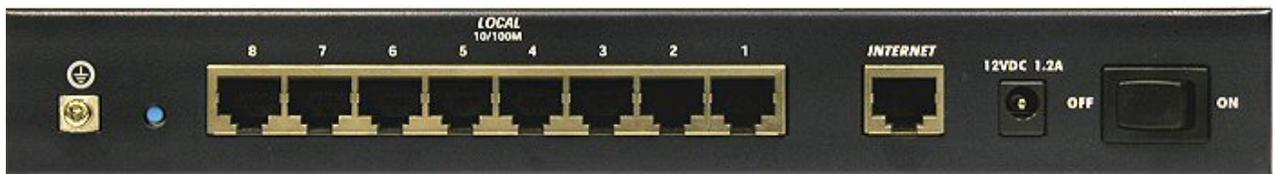
You notice that there is the one WAN port with 8 other Ethernet ports available for use. All routers have at least 2 IP addresses, always. One IP address is to connect to your ISP and is assigned to your WAN or Internet port and the other IP address is logically connected to all of the other 'switched' ports. For instance the WAN (public) IP from your provider could be 54.63.2.123 and the other IP for your LAN (private) may look like 192.168.x.x.
